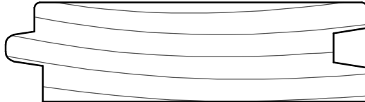
STG-09 3/4" x 2 23/32" (2 1/2" FACE DIM.) VARIABLE THICKNESS & WIDTH NON-STOCK
